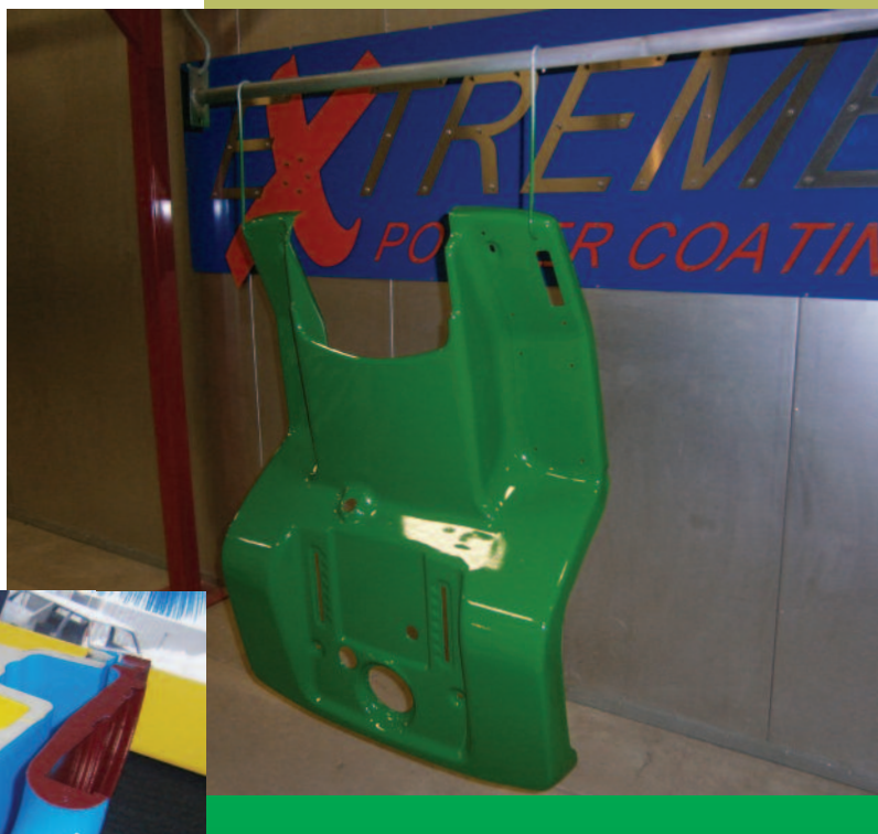
John Deere mower decking pieces are shown coated in Cardinal YL-01 and Diamond Vogel Tractor Green ET-6390.
